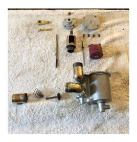
These are the parts of the carb The throttle is the bronze cylindrical part with the rectangular hole in it. This can be rotated inside of the smaller cylinder on the aluminum carb. The adjuster needle, which sets the mixture of gas and air, is in the same cylinder.
