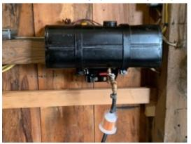
This is the ignition system. The coil is one of the two that I have. The points are the ones that I rebuilt installing new tunsten buttons. In the switch plate you see a SPST togle switch that is the rest ignition key. On the black disk you can see a strong spark jumping in the spark plug. I was very fortunate to find an original plug made in France for the Aster engine. The good news is that I can use a Model A Ford spark plug, like the one in the photo, when I install one in the engine.
