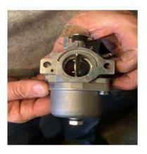
This is the carb that I have decided to try. After we get it running, I plan to insert an aluminum venturi into the original aluminum carb. I hope I can get the original carb to work well.
