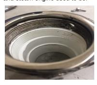
One of the parts that Frank was working on is a packing gland that attaches over the rear shaft and threads onto the crankcase.
