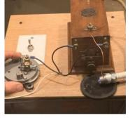
The next item for the test is the cooling system. I am using the type of pump that is used on a hot water, baseborad heating system in a house. These have worked well for me in the past.
