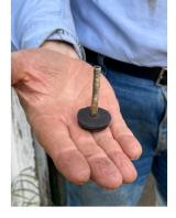
I have made a neoprene disk that will be the new seal in the carb. I will replace the leather seal with a fender washer to provide support for the neoprene.
