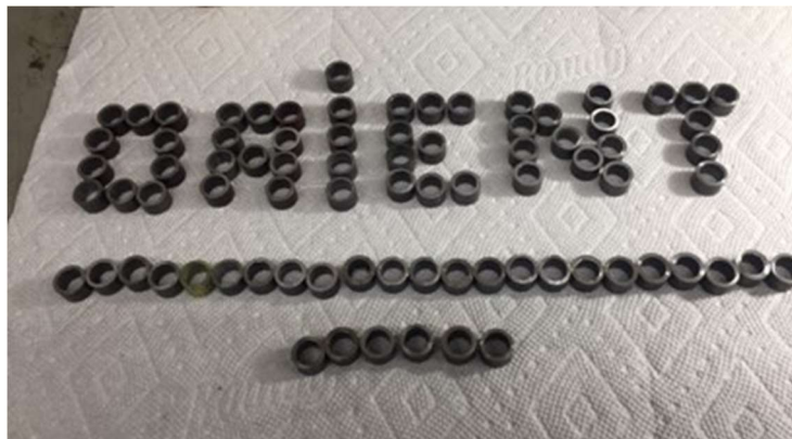
The reason that the chain did not fit properly on the sprockets is because the rollers are .625 in OD. We have determined that the proper size is .5625. Charlie made a tool to disassemble the chain links so we could remove the rollers and replace them with those of the correct size.
