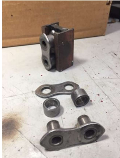
The reason that the chain did not fit properly on the sprockets is because the rollers are .625 in OD. We have determined that the proper size is .5625. Charlie made a tool to disassemble the chain links so we could remove the rollers and replace them with those of the correct size.
