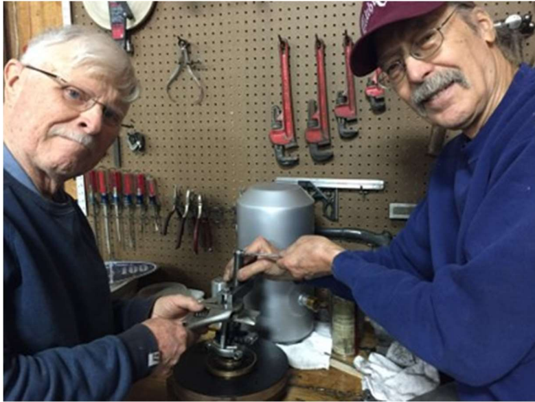
In this photo, Charlie and I are removing the small sprocket for the transmission drum. Charlie would machine the face of this sprocket to make it fit closer to the drum.
