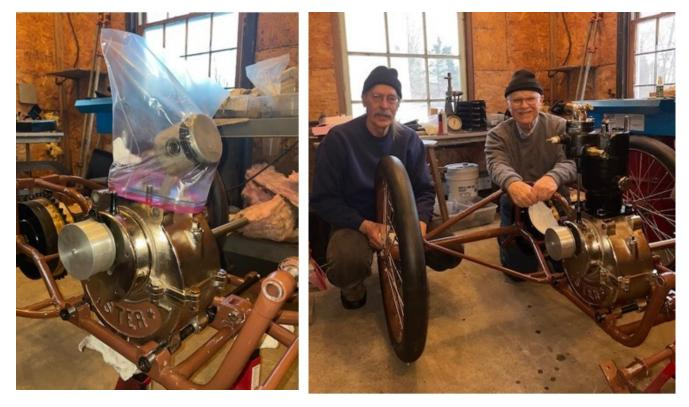
In the photo to left, I have attached the cover on the timer. This completes this end of this engine. The picture on the right was taken the day that Charlie came over and helped me put the cylinder on. We then put the head on which makes it look pretty good.
