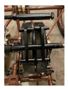
The photo to the left shows the transmission on the long shaft. Outside of the transmission you can see that bronze clutch control. To the left of that is a silver part which is a new bearing that I am currently working on to support the long shaft when the engine is running. To the left of the bearing is a cast iron ratchet which is attached to the shaft to start the engine with the starting crank that is outside of it.
