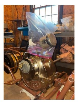
These photos show the piston mounted on the rod but before we placed the cylinder on it. In the first picture, I have mounted the drum that holds the gear from the crankcase and the gear (twice the diameter) that holds the cam and the push rod guide on top. The second photo shows the timer mounted to the cover of the drum. The small black piece of iron that is on top of the timer is what the spark lever attaches to from the steering column.
