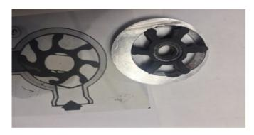
This is the new cylinder with the impeller. At this point, Frank tested the rotating the impeller and found it to be very difficult to turn. In fact, it would get more difficult to turn when we installed the cam to force the water out of the pump. This appeared to be a problem and my calculations proved that it was. The Jabsco pumps are used on marine engines over 300 horse power. They would have no trouble turning these pumps, but the loss of power from our 4.5 HP engine would not work.
