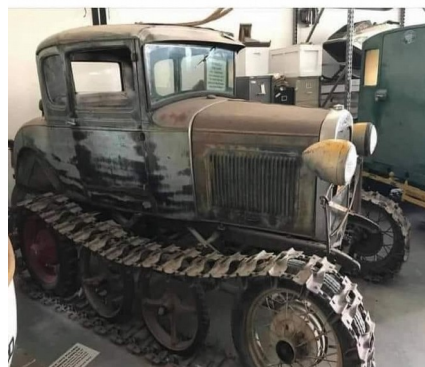
1930 Ford coup with "snowbird" track conversion. Used for delivering wintertime mail delivery in Montana way back when.
